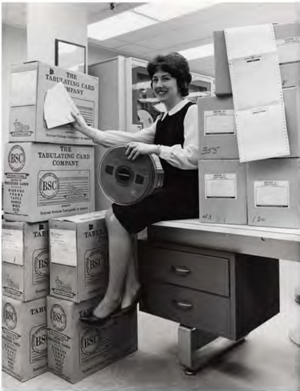
May 31, 1963 - More than 60,000 line items, as represented by these punch cards, are converted to 2,400 feet of magnetic tape on each of these two reels by means of the GE-225 computer system designed in Syracuse and now at use in General Electric's Nela Park. The result is the 5,500 customer invoices at the right.
