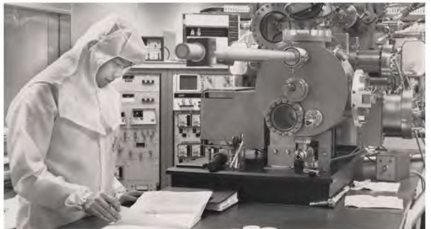
February 20, 1989 - GE Electronics Laboratory, Liverpool, Pin Ho, Senior Materials Engineer at the GE Lab... oversees gallium arsenide material growth on three inch wafers in the MBE reactor... the wafers are then used as the base for fabricating HEMTS, which require highly pure material for best performance...
