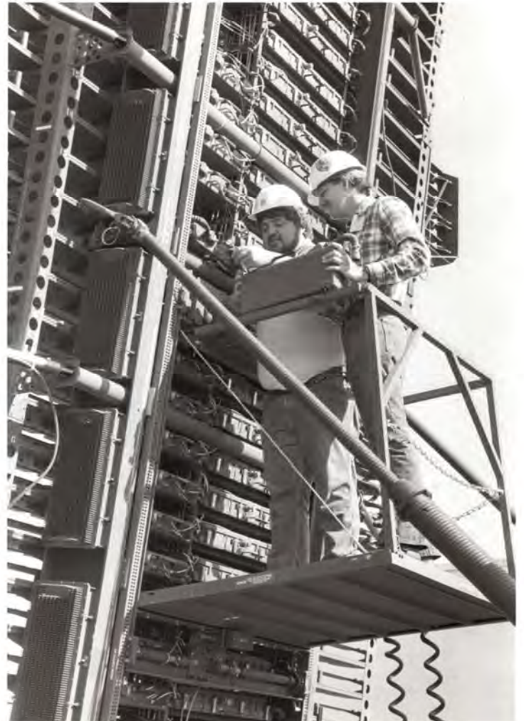
May 12, 1986 - This General Electric TPS-59 transportable radar is undergoing checkout prior to acceptance testing by the customer at General Electric's Electronics Park facility.
