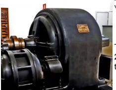
The **Driving Motor** is a 500 HP induction motor operating from a 2,200 volt supply. When the driving motor rotates at 711.3 rpm, the alternator produces the desired frequency of 17,200Hz.
