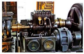
The **Gear Drive** increases the speed of the driving motor from 711.3 rpm to the alternator speed of 2115 rpm. This results in the alternator producing a frequency of 17,200 Hz.
